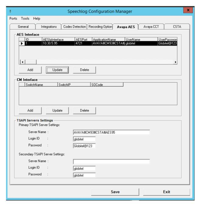
Enter the name of the Communication Manager for **Switch Name** and the IP Address of the Communication Manager server for **Switch IP**. The **SO Code** will not be used in this setup. Click on **OK** to continue.
