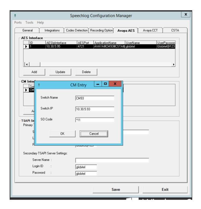
The **TSAPI Servers Settings** must now be completed, enter the Tlink information obtained from **Section 6.8** as the **Server Name**, the **Login ID** and **Password** are that of the AES user created in **Section 6.4**. Click on **Save** to save all the information just entered in this section.
