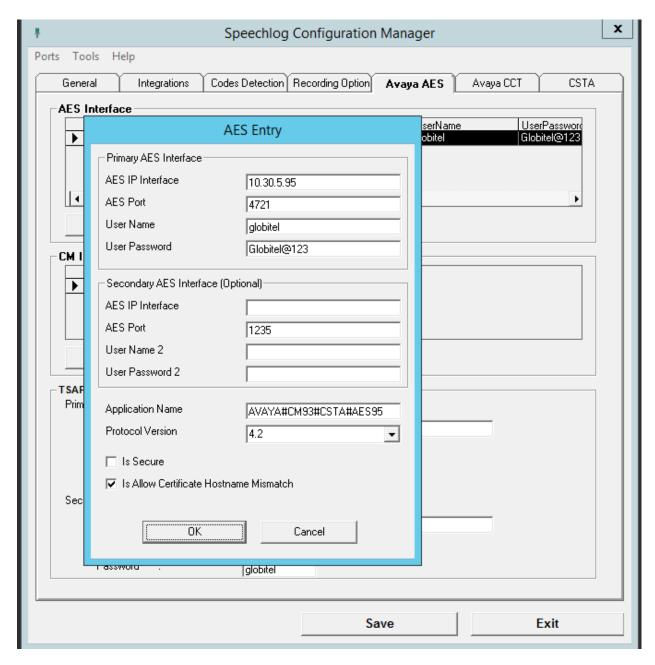
A new Communication Manager interface also needs to be added. Click on **Add** under the **CM Interface** section.
