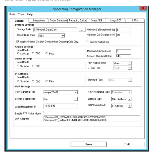
In order to complete the setup and place the recorder into service, the main recorder service should be stopped and started. Note that this may already be in a stopped state, if so simply start the service. If stopping and starting the service, allow a minute between these actions in order to allow all services to stop correctly before starting them back up again.
