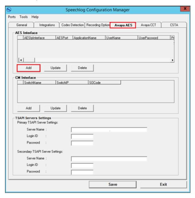
Enter the AES IP address for the **AES IP Interface** and the **AES Port** which should be the DMCC unsecured port number as shown in **Section 6.6**. The **User Name** and **User Password** is that which was configured in **Section 6.4**. The **Application Name** is the Tlink also secured from **Section 6.8**. The **Protocol Version** should be set to **4.2** and the tick boxes shown below should be ticked. Click on **OK** to continue.
