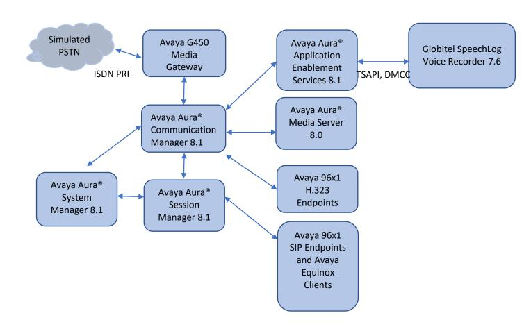
**Figure 1: Compliance Testing Configuration**
