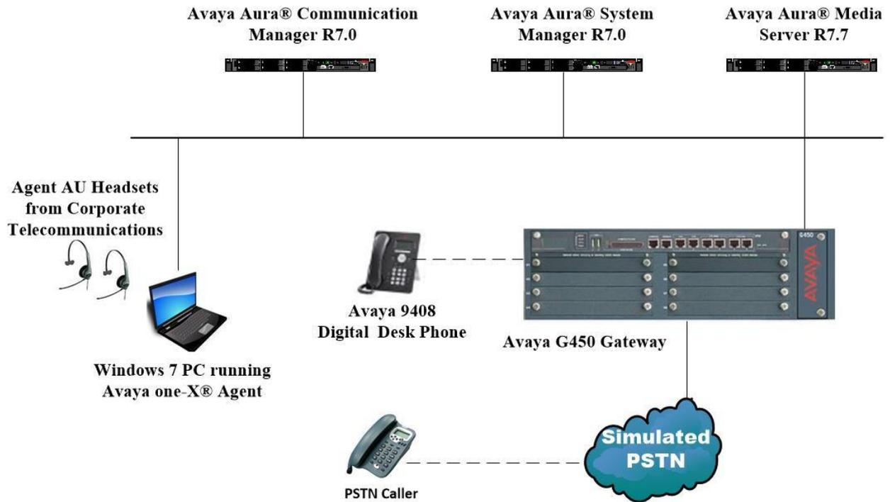
**Figure 1: Network Solution of the Agent AU Headsets from Corporate Telecommunications connecting to Avaya one-X® Agent**
