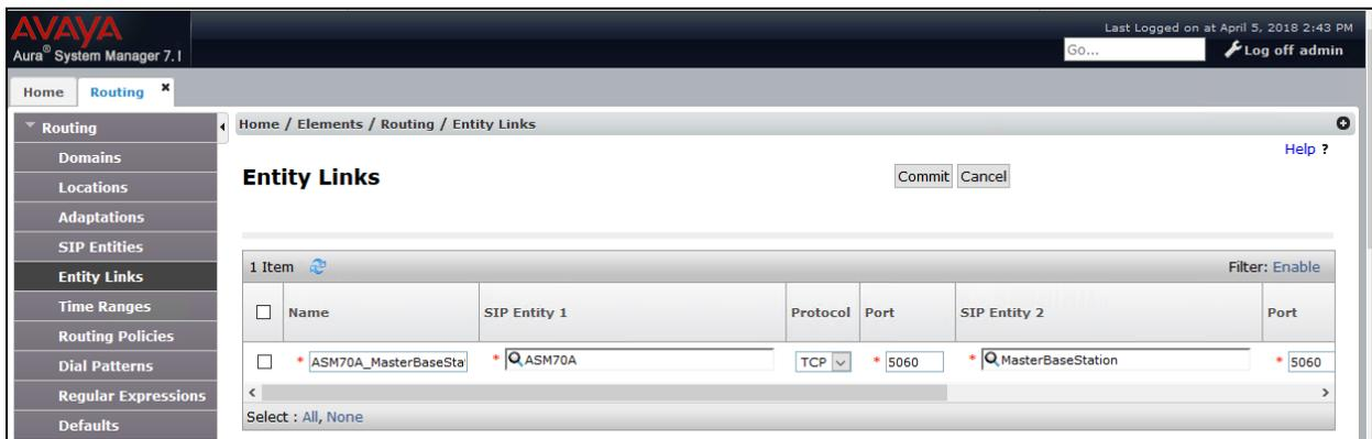
A SIP Entity and Entity link must be added for both the Ascom Master base station and the Ascom Slave (Standby) base station.
