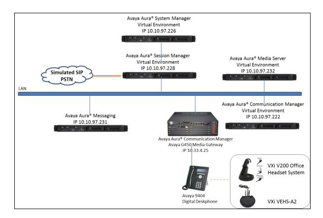
Figure 1: Test diagram for Avaya 9400 Series Digital Deskphone with VXi V200 Office Headsets and VXi VEHS-A2 EHS Cable.
