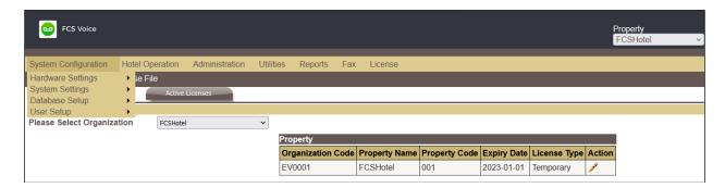
Click on the edit ('pencil') icon under **Action** and view the details. Ensure that the appropriate license parameters are enabled. Note that *Temporary* license was used for this compliance testing.
