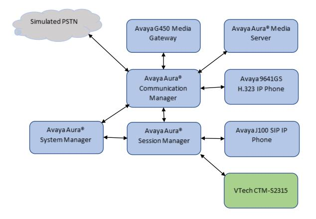
Figure 1: Avaya Test Configuration for VTech CTM-S2315
