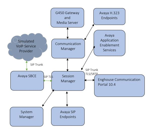
Figure 1: Test Configuration for Enghouse Communication Portal and the Avaya Platform.
