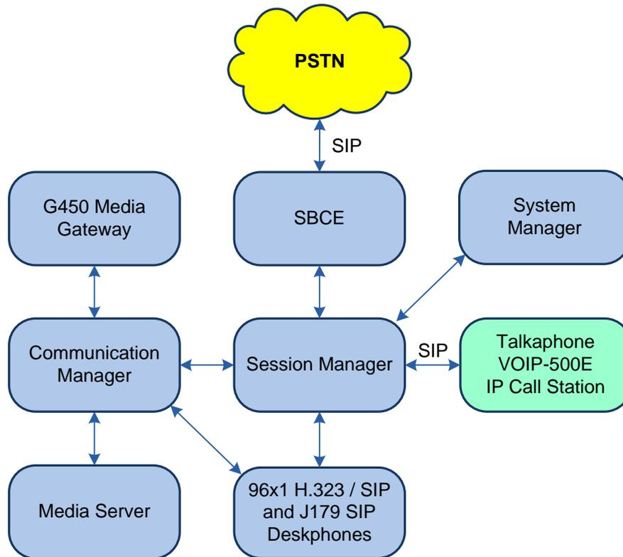
**Figure 1: Avaya SIP Network with Talkaphone VOIP-500E IP Call Station**
