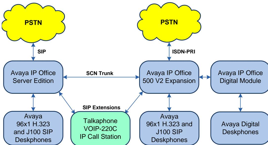
**Figure 1: Avaya SIP Network with Talkphone VOIP-220 Series IP Call Station**
