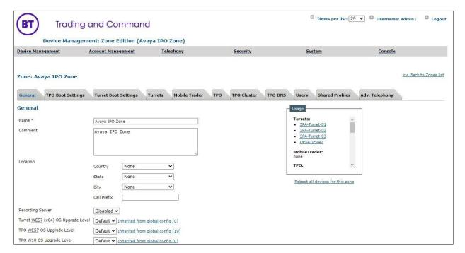
Navigate to the **Turret Boot Settings** tab in Avaya IPO Zone, then select **SIP** option **Basic Mode** and update Avaya IP Office server address to 10.128.226.178 and other highlighted parameters below.
